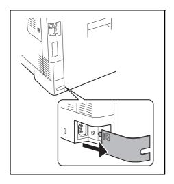
3 Remove the Power Cord Connector Cover.
